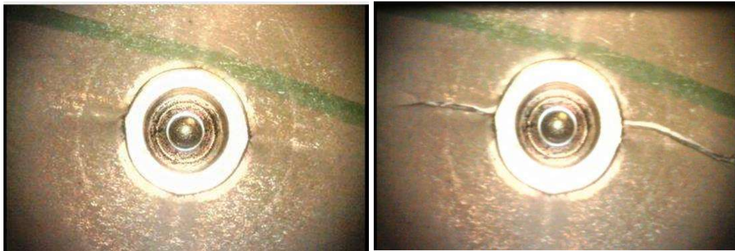
Figure 4: XPF1000 in a flat nosed punch test, just before and just after fracture
